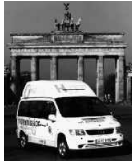
Mercedes's new hydrogen-fuelled NECAR II minivan pictured at the Brandenburg Gate, Berlin. The compressed-gas tanks are on top.
