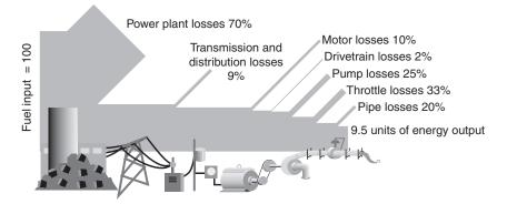
**FIGURE 1** To deliver one unit of flow in the pipe requires about 10 units of fuel at the power plant, thus those 10-fold compounding losses can be turned around backward, yielding 10-fold compounding savings of fuel for each unit of reduced friction or flow in the pipe. From the E SOURCE "Drivepower Technology Atlas," courtesy of Platts Research & Consulting.
