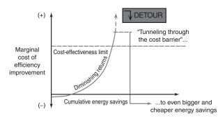
**FIGURE 3** Optimizing whole systems for multiple benefits, rather than isolated components for single benefits, can often "tunnel through the cost barrier" directly to the lower-right-corner destination, making very large energy savings cost less than small or no savings. This has been empirically demonstrated in a wide range of technical systems.
