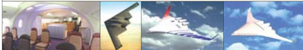
Figure 26: Next-generation airplanes. L-R: Interior view of Boeing's mostly-composite long-range 7E7 Dreamliner, to enter service in 2008 with 15–20% fuel saving at no greater cost; Northrop flying-wing B-2 bomber, showing how the low-signature engines of a Blended-Wing-Body design can be packed inside; artist's conception of a civilian BWB airplane without this potentially efficiency-improving feature; 405 and an artist's conception of a civilian BWB with ultra-efficient engine technology, embedded wing propulsion, and boundary-layer ingestion engine inlets with active flow control.
