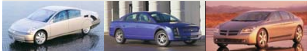
Figure 10: Three 2000 PNGV 245 diesel-hybrid midsize concept sedans and their gasoline-equivalent mpg L to R: GM Precept (1,176 kg, C_d 0.163, 80 mpg), 246 Ford Prodigy (1,083 kg, C_d 0.20, 70 mpg), 247 and Dodge ESX3 (polymer body, 1,021 kg, C_d 0.22, 72 mpg). Of their efficiency gains, totaling 2.7–3.1× vs. the 26-mpg Taurus -class base vehicle, ~15–18% came from switching to diesel engines, 36–47% from smaller loads and engines (better platform physics, accessories, and their consequences), and 43–48% from hybridization. 248 ESX3 's cost premium over a Chrysler Concorde at 80,000 units/y was cut from the initial 1996 ESX 's $60,000 to $7,500, equivalent to a ~$28,500 MSRP. 249 However, none of these concept cars has yet been turned into a market platform due to their higher production cost, which is ascribed largely to costlier light metals and greater powertrain complexity.
