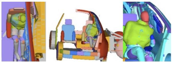
Figure 7: UltraLight side impact simulation at 20 milliseconds (TASS)
