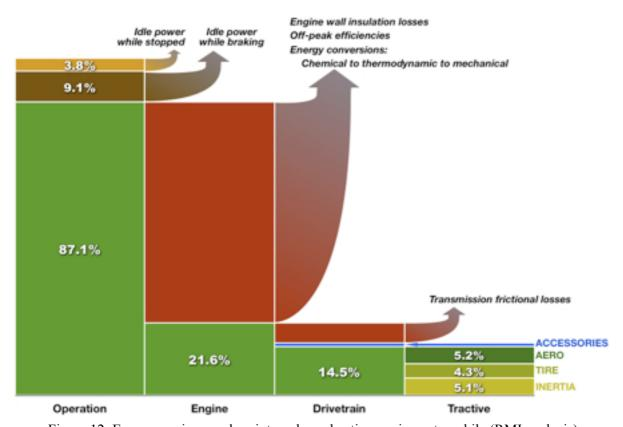
Figure 12: Energy use in a modern internal-combustion engine automobile (RMI analysis)
