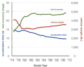
Figure 1: Light-duty vehicle performance and weight (U.S. EPA; 3-year moving average)
