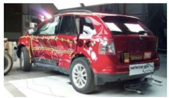
Figure 6: 2007 Ford Edge after side impact crash test (NHTSA)
