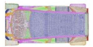
Figure 5: Revolution frontal-impact simulation during maximum crush at 54 milliseconds (TWR Engineering)
