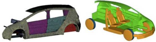
Figure 3: UltraLight Finite-element model, left, and ellipsoid multi-body model in orange, right (TASS)
