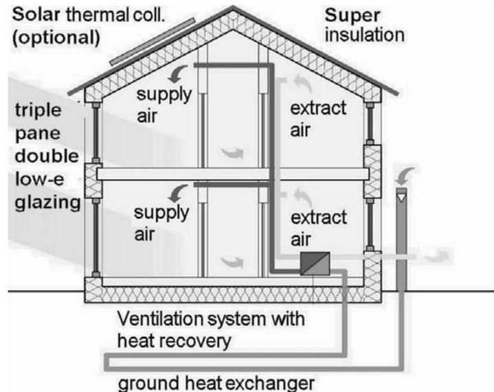
*Figure 1 Passivhaus building section showing typical systems.*
