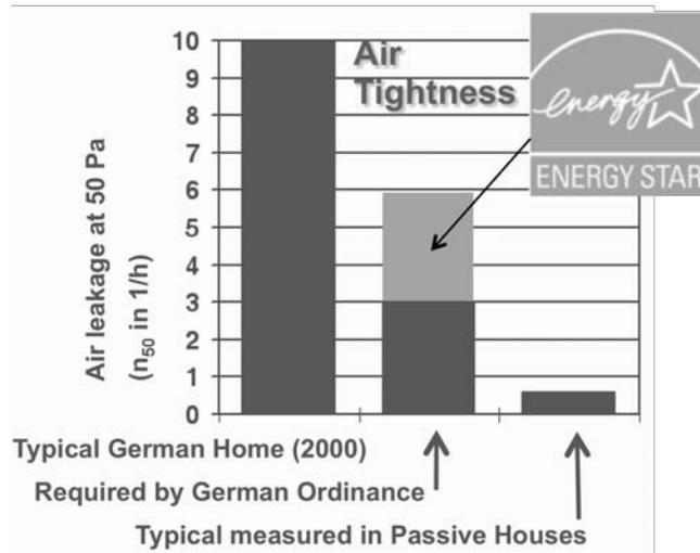
**Figure 2** Relative air tightness of typical German home, Energy Star, and Passive House.
