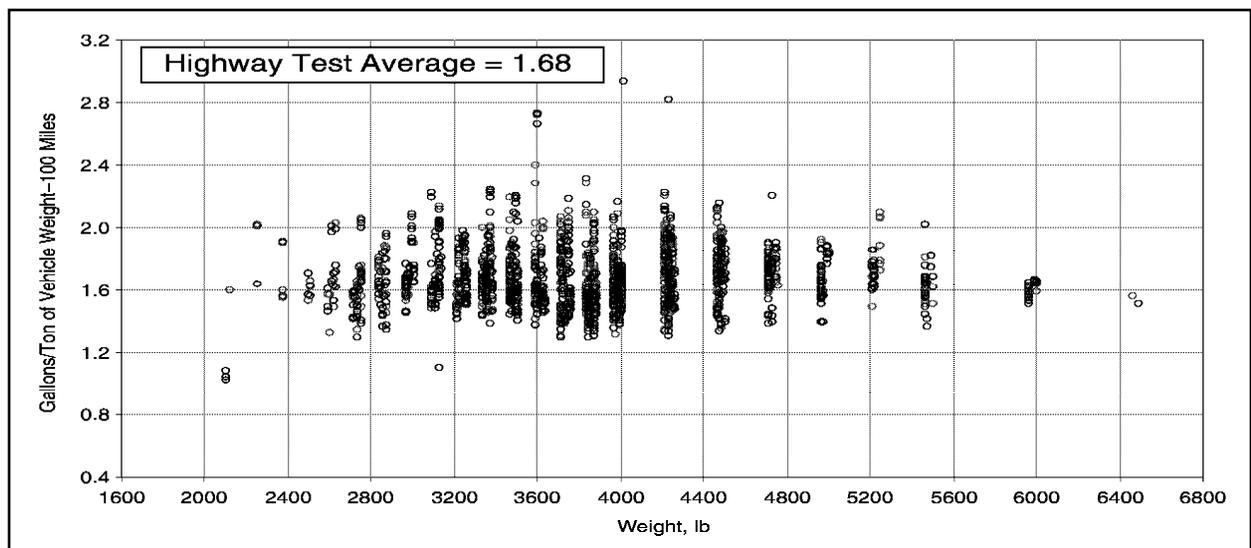
vehicle model in the MY2000–01 U.S. new-light-vehicle fleet.<sup>33</sup> Note the large vertical scatter at a given weight.
