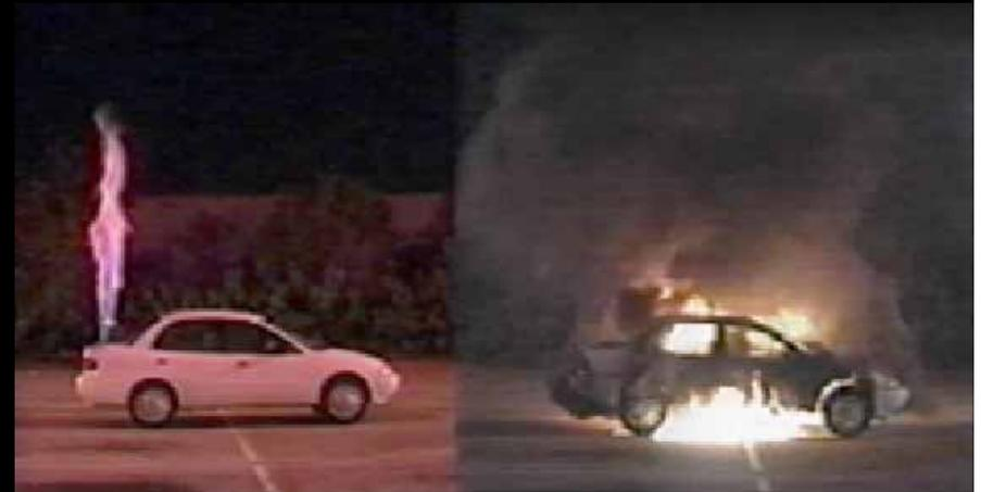
60 s: H<sub>2</sub> flow subsiding; max 47°C on rear window, 19.4°C on tray behind rear seat. Zooming in on gasoline car...
