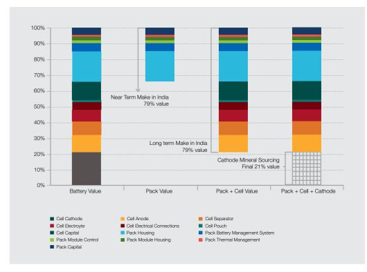
Figure 9. India can quickly capture 25–40% of component production cost of Lithium-ion batteries by assembling packs in India. It could capture almost 80% of this value over time. Source: Bloomberg New Energy Finance, Bottom-Up Cost Scenarios for Li-ion Batteries 70, February 2017, and NITI Aayog and RMI analysis
